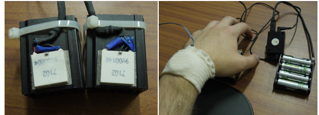
Figure 1: Peltier modules used to produce thermal stimuli (left); experiment apparatus with Peltiers under palm (right).
